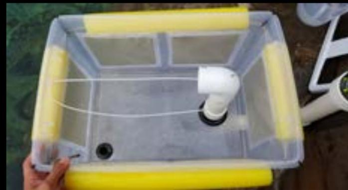
Figure 2. Internal view of an air driven egg collector designed and built for this project.
